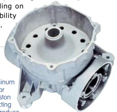
An all-aluminum frame, motor housing, piston and connecting rod help to reduce thermal stress and help the compressor run cooler by dissipating heat away from the bearing surfaces.
