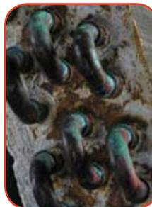
Copper tube and galvanized steel tube sheet after 500 hour salt spray.
