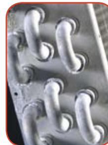
Aluminum tube and tube sheet after 500 hour salt spray.
