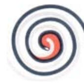
**Hot, High Pressure—Discharge Gases.** As the spiral continues to orbit, the gas is compressed into an increasingly smaller pocket. By the time the gas arrives at the center port, discharge pressure has been reached.
